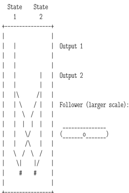
The paths here are smoothly curved channels in the plane. An oblong “follower” with rounded ends begins in either the State 1, Output 1 or State 2, Output 2 position at the top of the diagram, and
