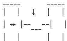
The transverse displacement is relatively large (much larger than the displacement that would have been transmitted to the driven block) and oscillating, but the transverse force need do no net work over time. Consequently you want to apply this displacement through a spring with high compliance.
