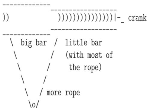
This is going to put rather significant side forces on the rope that will attempt to slide it along the length of the bar, add extra tension to the rope that isn't part of the load it's bearing, and change the mechanical advantage.
