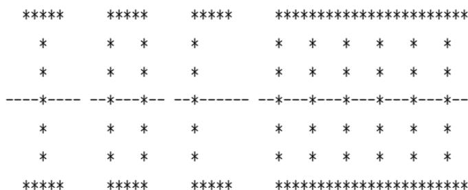
(This kind of sandwich panel, a single plastic with square channels running through it, is in common use for translucent roofing for bus stops around here; it’s called “twinwall plastic” when made from polycarbonate, and similar sandwich panels made from other plastics are called “corrugated plastic”, “corriboard”, or “coroplast”.)
