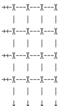
Here each of the "X" points is a switch which can either transmit a signal from the input to the output, or not, according to the switch configuration, and each of the "↓" is an output register consisting of 16 D flip-flops which registers the input that has been routed to it. An example configuration, with "+" indicating switches that are disconnected and "#" indicating those that are connected, follows:
