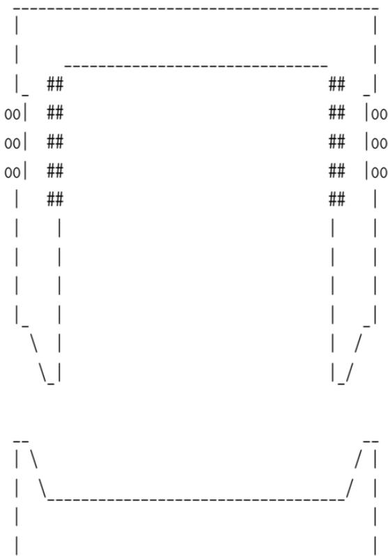
With this arrangement, when the contents overheat and melt into the bottom of the kiln, they destroy only the bottom plate, which is the easiest part to replace; and, of the electrical components, only the inexpensive steel pipe is exposed to the high temperatures inside the kiln. The copper windings, in particular, are insulated from the pipe by a significant thickness of refractory material.
