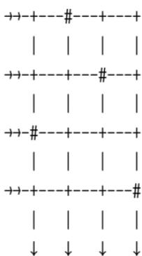
(With some logic families, it might be appealing to double that to 16 bits of configuration data instead of 4 and get wired-AND or wired-OR functions between the inputs, plus a free all-zeroes or all-ones value, depending on whether it's AND or OR.)
