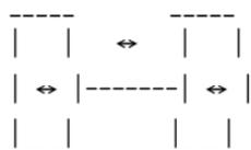
However, a relatively small force pushing on the side of the rod can get it to buckle when it otherwise wouldn't, greatly reducing the force transmitted to the driven block:
