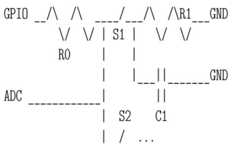
Your GPIO pin, a switchable voltage source, connects through a resistor  $R_0$  to a common bus to which all the pushbuttons connect. Your ADC is also connected to this common bus. Each pushbutton  $S_i$  connects the bus to a resistor  $R_i$  and a capacitor  $C_i$ , each of which is grounded on the other side; that is to say, they’re in parallel.
