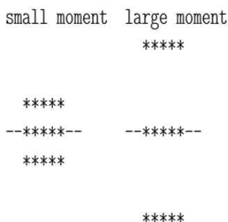
The trouble with this is that once we insert empty spaces in the middle, it stops being a solid object. We need to put enough stuff in the middle to keep the parts moving together; the stuff in the middle is pretty much only stressed in *shear*. Also, when the column is flexing, the facesheet on the inside of the bend is in compression merely from the flexing, and that compression can cause *it* to buckle.
